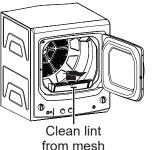
**Dryer Interior and Duct:** The interior of the appliance and exhaust duct should be cleaned once a year by qualified service personnel.
