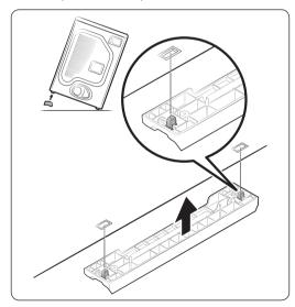
STEP 4 Bottom view of the dryer after assembling the Stacking Support Guides to the dryer base.
