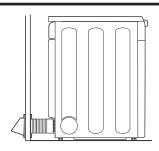
DO cut duct as short as possible and install straight into wall.
