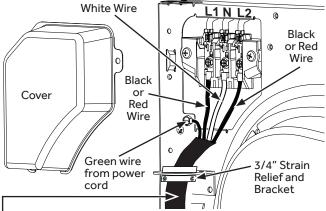
4 #10 AWG minimum copper conductors or 120/240V 30A power supply cord kit marked for use with dryers and provided with closed loop or spade terminals with upturned ends (not supplied).
