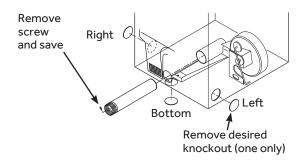
Detach and remove the right, left or bottom knockout as desired. Remove the screw inside the dryer exhaust duct and save.
