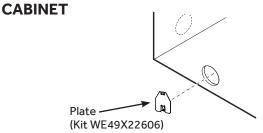
Connect standard metal elbows and ducts to complete the exhaust system. Cover back opening with the plate (kit WE49X22606) which can be purchased from haierappliances.com/parts or in Canada visit haiercanada.ca/parts. It may also be obtained from a local service provider. Place dryer in final location.
