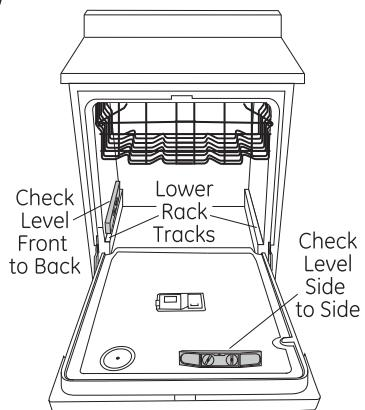
If your model has a rear leveling system, the rear height is adjusted from the front of the dishwasher along with the 2 front legs on the bottom of the dishwasher. Begin the leveling process with the front legs by individually turning the front 2 legs. Adjust the front legs first. When the front legs are adjusted to a height resulting in an appropriate gap to the upper cabinet, proceed to adjust the rear leveling system by adjusting the leveling bolt as illustrated in the figure.
