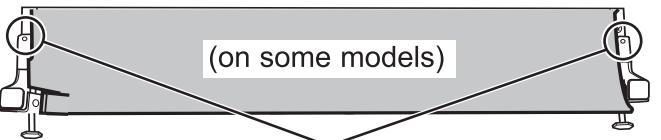
Push the sides of the insulation behind the toekick attachment screw holes
