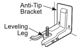
drawer or kick panel can be removed for easy inspection. If visual inspection is not possible, slide the range forward, confirm the anti-tip bracket is securely attached to the floor or wall, and slide the range back so the rear leveling leg is under the anti-tip bracket.
