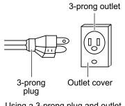
Using a 3-prong plug and outlet
