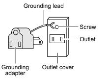
Using a grounding adapter
