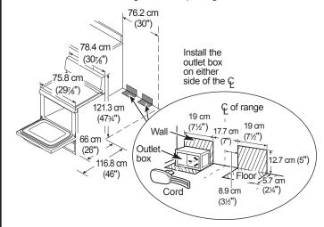
NOTE: Use a 1.2 m (4') power cord to prevent interference with the storage drawer. Power cords 1.4 to 1.8 m (4½' to 6') long may have to be dressed to allow for proper drawer closing.
