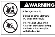
All ranges can tip. BURNS or other SERIOUS INJURIES can result. INSTALL and CHECK the ANTI-TIP bracket following the instructions supplied with the bracket.
