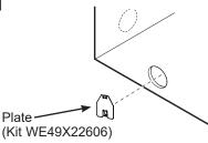
Connect standard metal elbows and ducts to complete the exhaust system. Cover back opening with the plate (kit WE49X22606) which can be purchased from **GEApplianceparts.com** or a local service provider. Place dryer in final location.
