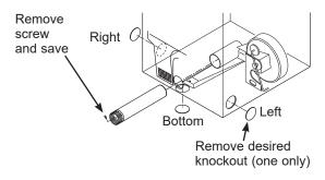
Detach and remove the right, left or bottom knockout as desired. Remove the screw inside the dryer exhaust duct and save.
